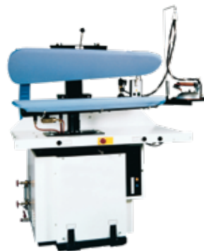
FPA1-D Automatic Cleaning Press with universal shape
